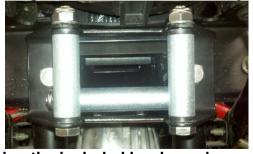
5. Secure your winch using the included hardware in your winch kit. Wire the winch according your manufacturers specifications. Mount your contactor on the inside of the firewall, you may need to swap the long cables and short cables to reach the battery. Always remove the negative battery terminal when working with vehicle electronics.
